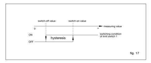
With limit switch 1 set for flow rate and a flow volume/time unit selected in menu DISPLAY SELECT, and when setting the switch-on and switch-off value, the pertinent flow volumes will also be indicated.
