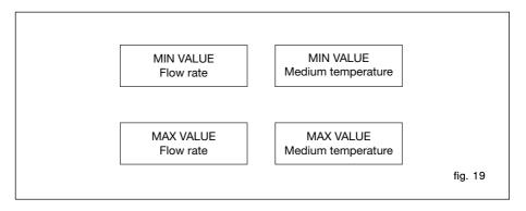
After switch-on or NOT-BUSY indication, the minimum and maximum values are deleted and will be continuously updated (non-return pointer principle).
