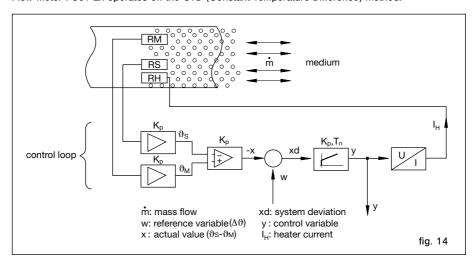
The temperature difference  $\Delta$  between the two sensors is kept constant and the mass flow is determined by measuring the calorific power.
