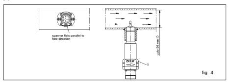
With inner pipe diameters of > 56 mm the middle of the probe (chamfer) must be screwed in to 1/8 of the inner pipe diameter.
