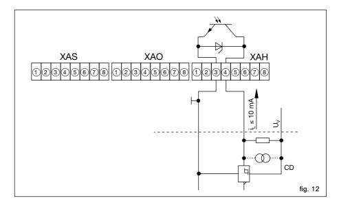
The quantity-dependent pulse to operate a counter or higher-order control is available at connector XAH /BUSY E/- and /BUSY C/+ (pins 3 and 4) (see fig. 11 - Circuit diagram FC01-Ex - open collector output).
