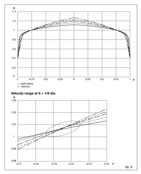
Max. accuracy is achieved with an insertion depth of x = 1/8 inner pipe dia. (fig. 7).
